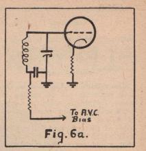
constant following the same laws as previously explained. It is desirable to include the resistances in the circuit to prevent undesirable coupling between the R.F. and I.F. stages which may produce instability.
