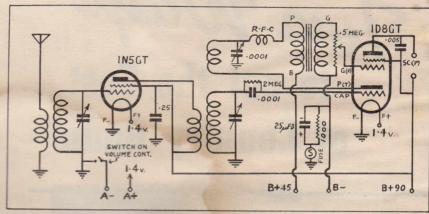
The schematic diagram of the circuit. which means such battery economy.
