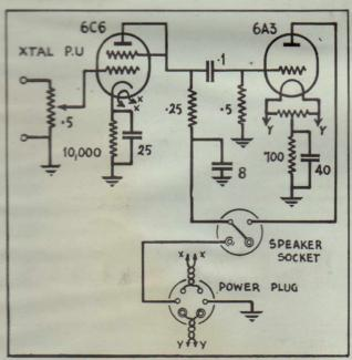
Here is the circuit diagram, showing that the design is conventional, and the exceptional performance is obtained by keen attention to detail.
