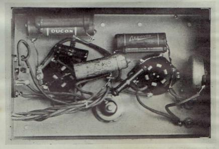
from the two fat pins of the plug are for the filament of the 6A3, and so these go to the lugs for the two fat holes of the four-pin socket, with the small centre-tapped resistor soldering on to these lugs at the same time.
