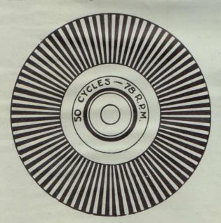
By cutting out this diagram and pasting it on to a piece of cardboard you can make a stroboscope which will let you check the speed of your turntable, while the record is actually playing.
