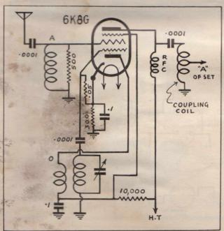
Schematic diagram of the circuit, showing the simplicity of the arrangement. A single-gang condenser does all the taning and no alignment adjustments are required.
