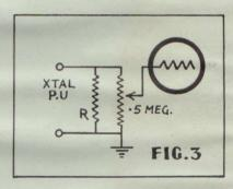
Diagrams showing various ways of changing the loading for a crystal pick-up to change the frequency response. Fig. 1 shows a way of retaining brilliance at low volume levels. Fig. 2 shows how to make the load adjustable. Fig. 3 shows how a quarter or half meg, resistor should be fitted if the low notes are too boomy.
