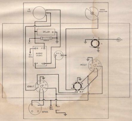
The picture diagram of the wiring.
