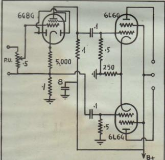
Circuit of the amplifier showing the simple phase changer and audio amplifier valve.
