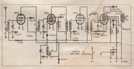
The circuit diagram showing the automatic biassing arrangement.
