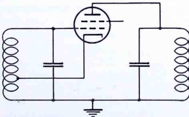
Fig. 13—Oscillator circuit employing positive current feedback
