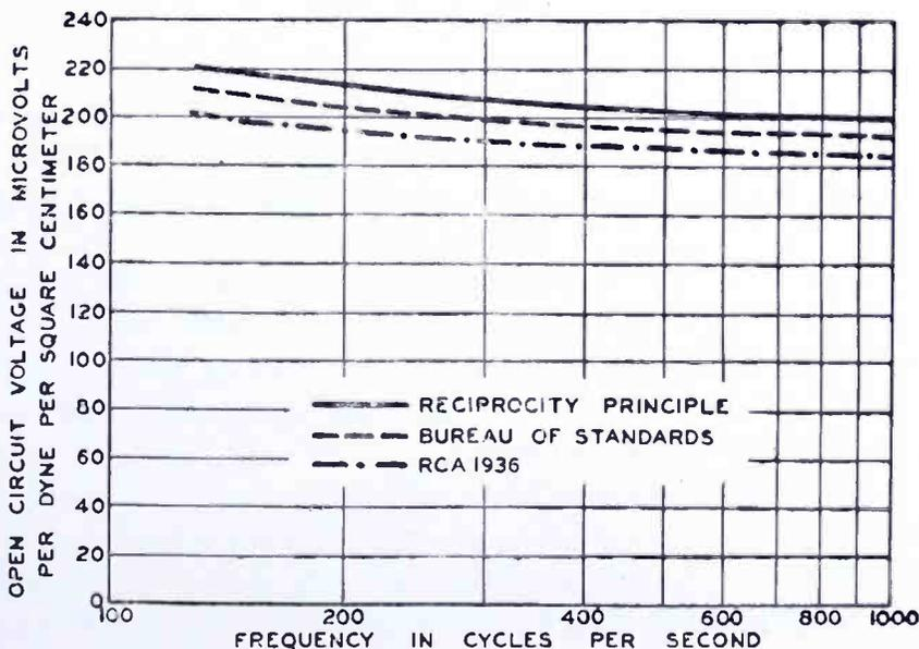
Fig. 4—The open-circuit voltage response vs. frequency characteristics at the 250-ohm output terminals of a commercial-type velocity microphone for a free field pressure of one dyne per square centimeter.
