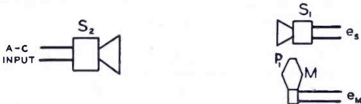
Fig. 2—Arrangement for obtaining the ratio of the open-circuit voltages  $e_M$  and  $e_S$  of the microphone  $M$  and the microphone-loudspeaker  $S_1$  when actuated by the same sound pressure  $p_1$  produced by the loudspeaker  $S_2$ .
