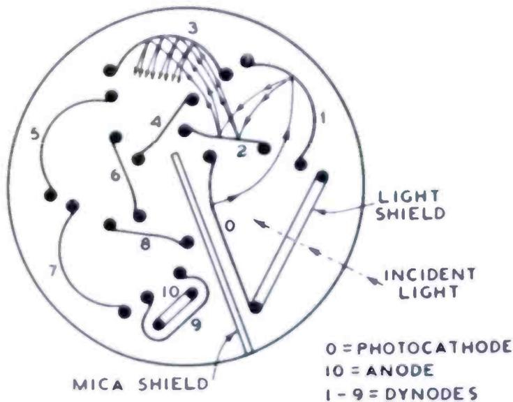
Fig. 7—Internal structure of the 931.
