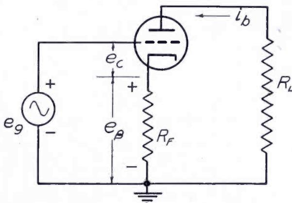
Fig. 6—Negative current feedback
