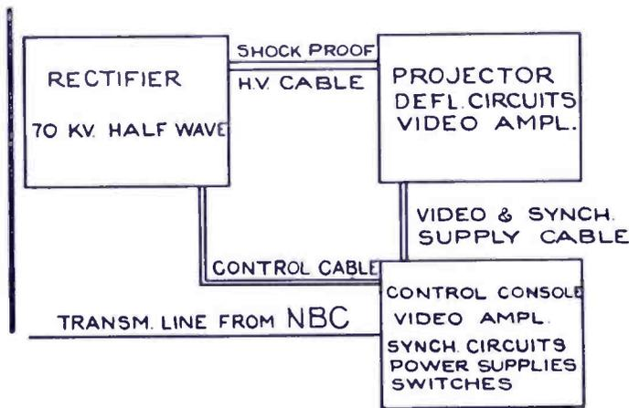
Fig. 5—Block diagram of the installation in the New Yorker Theatre.
