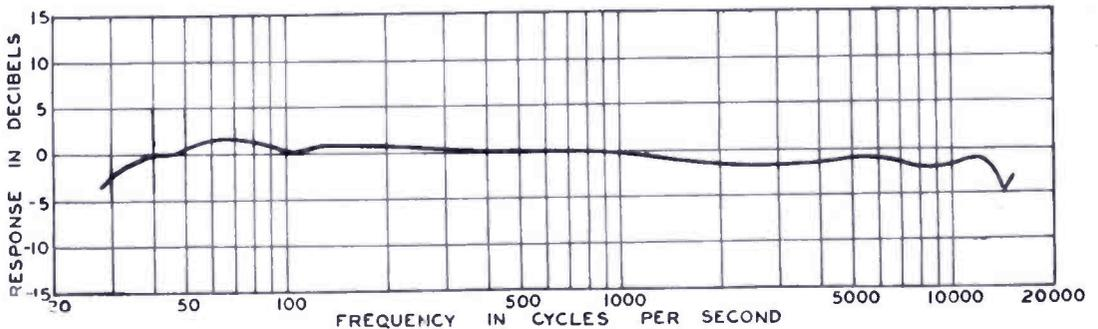
Fig. 5—The open-circuit voltage response vs. frequency characteristic at the 250-ohm output terminals of a commercial-type velocity microphone obtained by the principles of reciprocity and similarity. 0 db = 200 microvolts per dyne per square centimeter.
