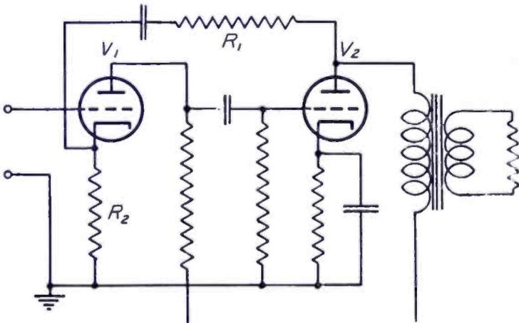
Fig. 14—Feedback over two stages
