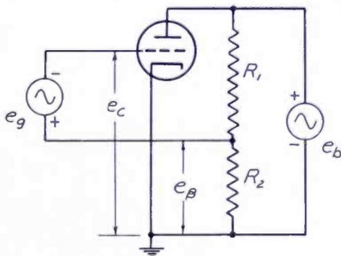
Fig. 1—Negative voltage feedback
