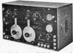
The panel is of Bakelite-dilecto. The coils are bank-wound inductances, of high frequency cable wound on threaded Bakelite-dilecto tubes, impregnated and baked.
