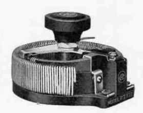
R EHOSTAT, Model PR-535, consists of a moulded base, approximately  $2\frac{1}{2}$  in. in diameter, on which are secured two concentric windings held securely in place by clamping screws. Connection is made to these windings by means of two sliding contacts of phosphor bronze, which form a circuit between the outside and inside windings. They are so shaped as to make continuous contact with at least two turns of wire, thus reducing tube noises during adjustment.
