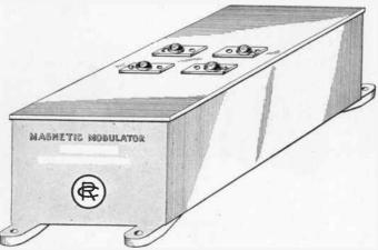
it is an ideal modulation device for purposes requiring the control of radio frequency energy at short wave lengths, such as is demanded in amateur radio telephony.
