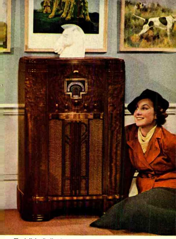
Magic Voice Radio 10-K: Magic Brain, Magic Eye, Metal Tubes. 150-410 and 530-60,000 kcs. Magnificent console-model Superheterodyne of 10 tubes, 5 bands. A wealth of every type of broadcasting, beautifully reproduced with higher fidelity with such features as 12<sup>th</sup> Super-fidelity Speaker, Higher Fidelity selectivity control, full Automatic Volume Control, and Automatic Tone Compensation, Music-Speech Control.
