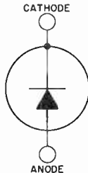
The arrow indicates direction of forward (easy) current flow as indicated by dc ammeter.
