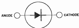
The arrow indicates direction of forward (easy) current flow as indicated by dc ammeter.
