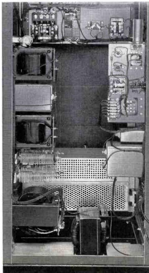
The lead between the modulator and modulated 4X250B grid contains an r-f trap. In the TTL-100AH this trap consists of a quarter-wave stub "shorted" at the end opposite the grid by a capacitor. Looking toward the modulator from the grid, the r-f sees a high impedance. The stub is resonant at approximately channel 10, but is effective from channel 7 to 13 without adjustment.
