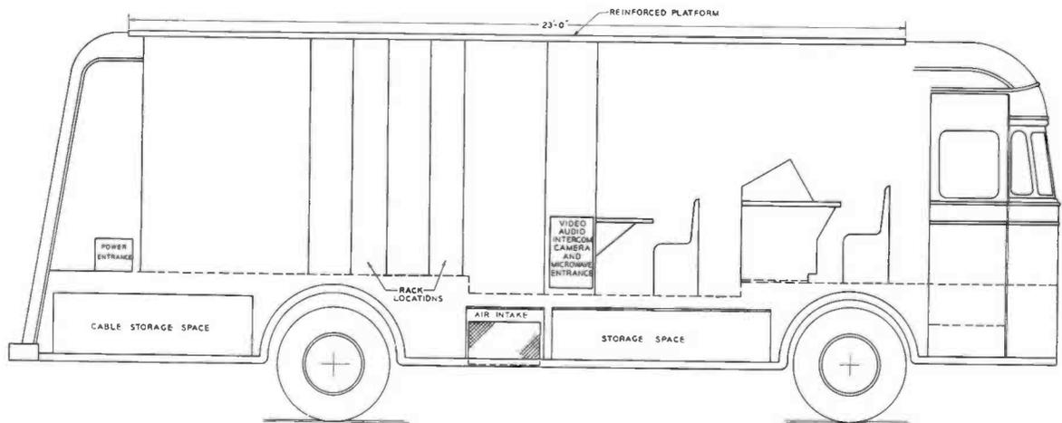
FIG. 6. Side elevation view of mobile control room.
