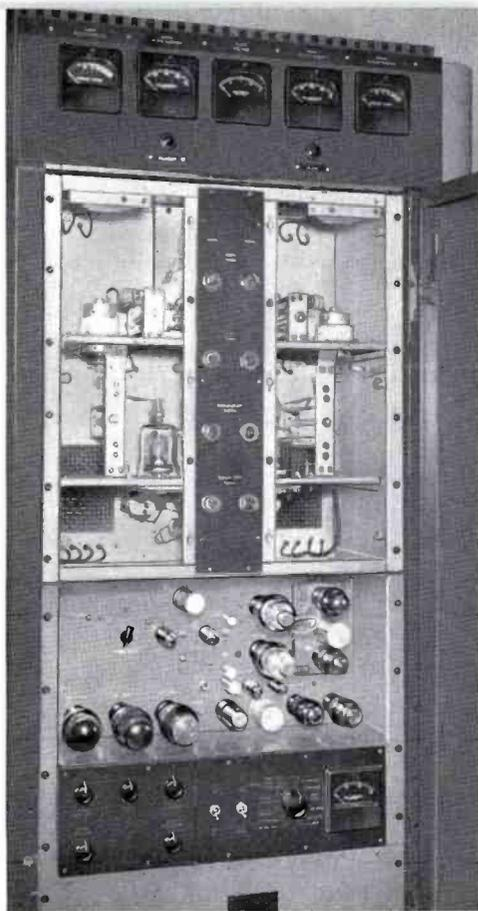
FIG. 3. Open view of the TTL-100AH VHF TV transmitter showing aural visual r-f cubicles, and modulator chassis and control panel mounted below.
