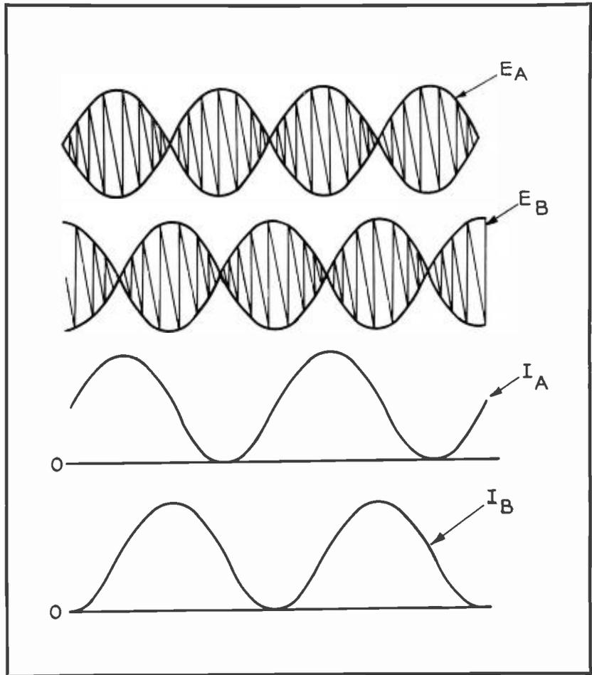
FIG. 11. Waveforms of stator output signals.
