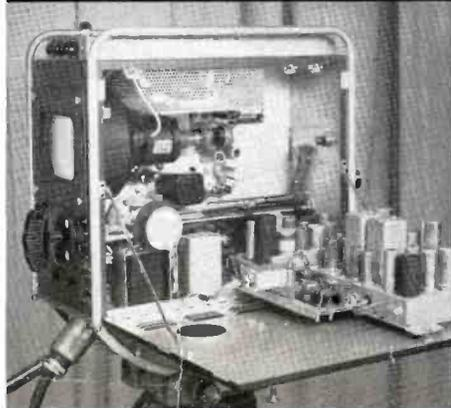
CAM OPERATED FOCUS MECHANISM
