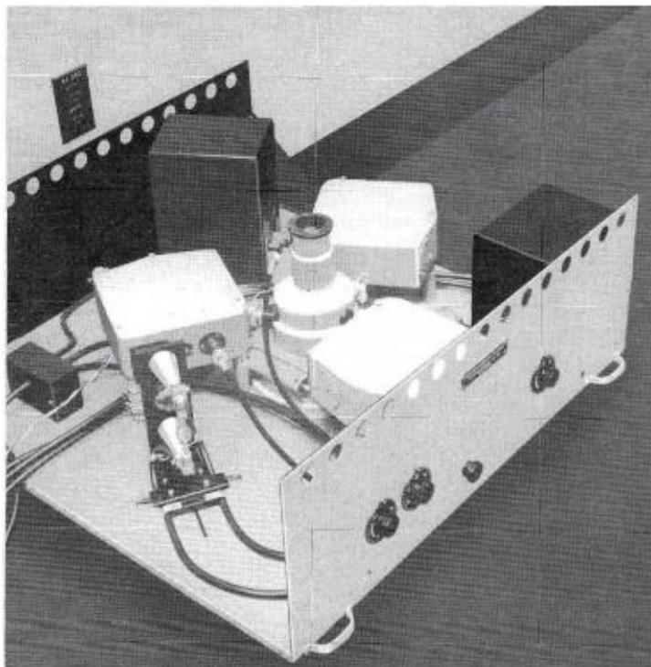
FIG. 4. Illuminating system for Ultraviolet Color-Translating Television Microscope.
