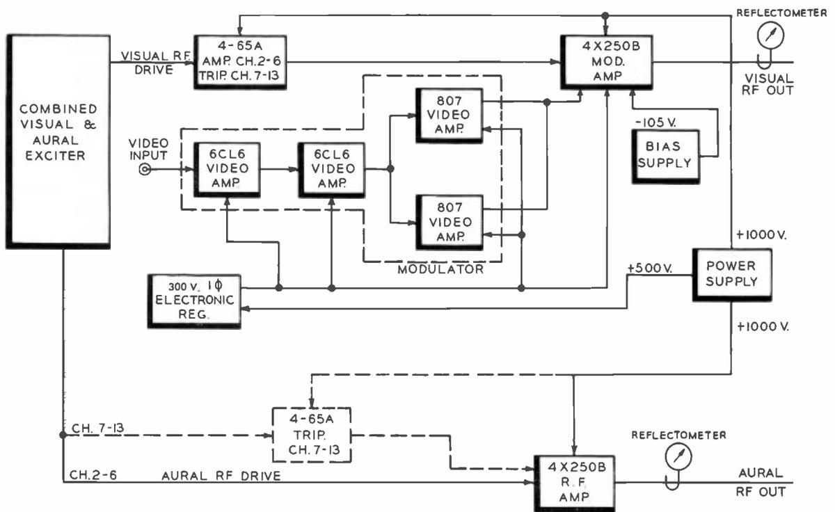
FIG. 2. Simplified block diagram of the TTL-100AL/AH Transmitter.
