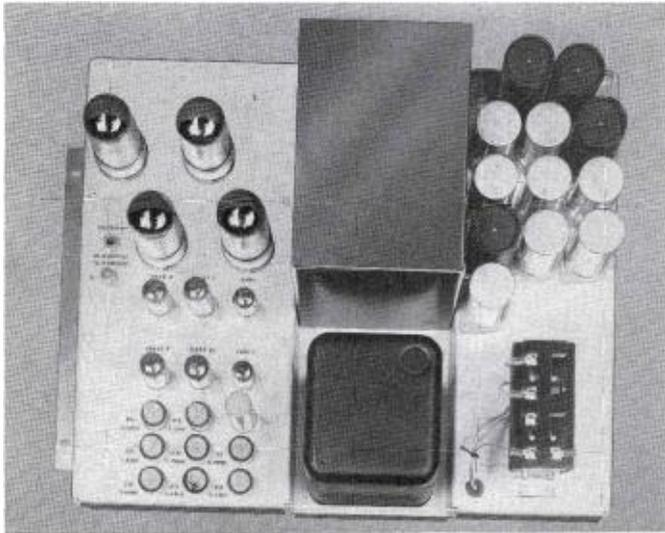
FIG. 17. Three-in-one power supply chassis.
