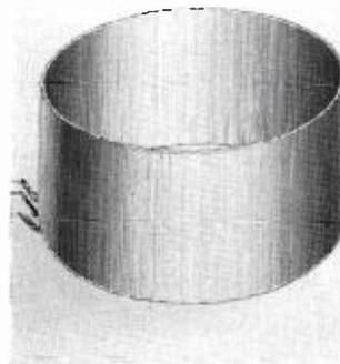
FIG. 8. View of the orbiting coil used with electromagnetic orbiter.
