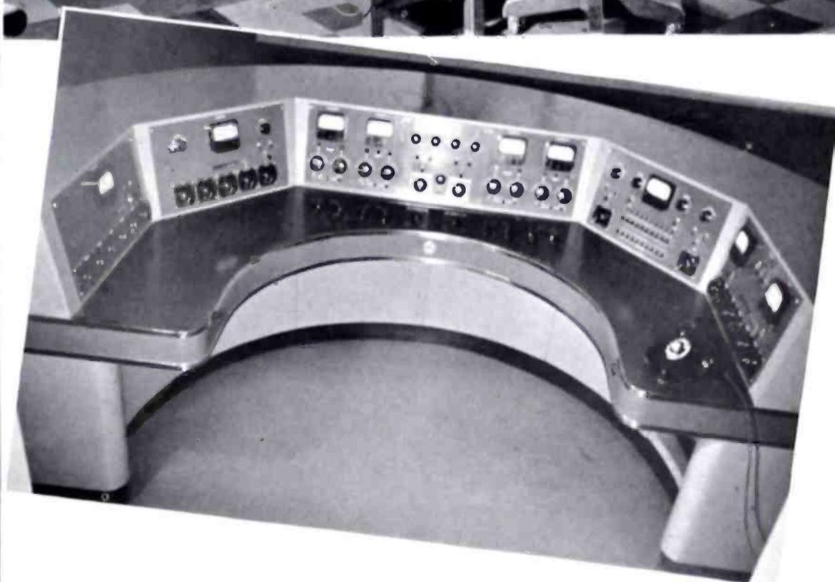
▲ The RCA Custom Built Speech Input Control Desk at WTAG. Control panels are included for 3 studios and switching. "Preset" facilities for 4 outgoing lines are provided. The second panel from the right contains equipment for remote line switching and equalization.
