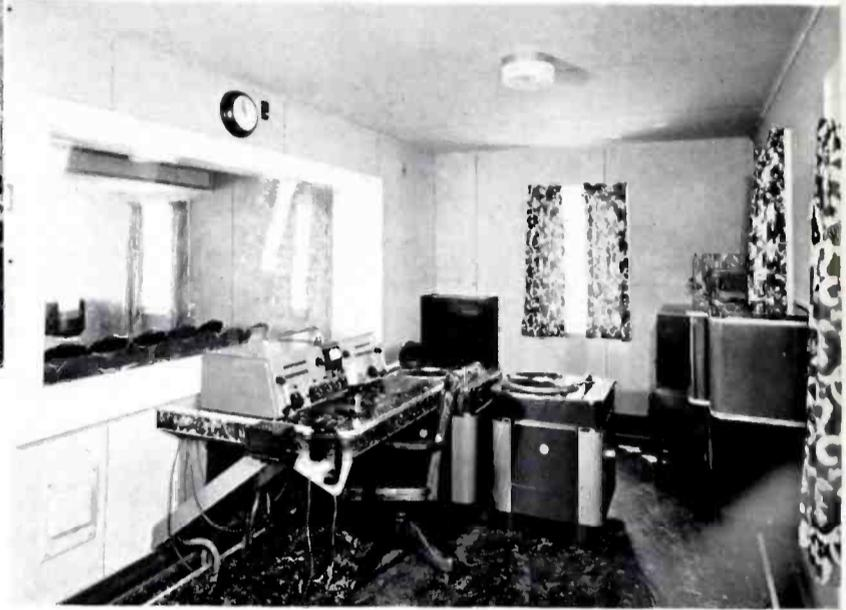
▲ RCA 76 B Console, 70-C Turntables and 64-B Loudspeaker are combined to provide an efficient speech input system.
