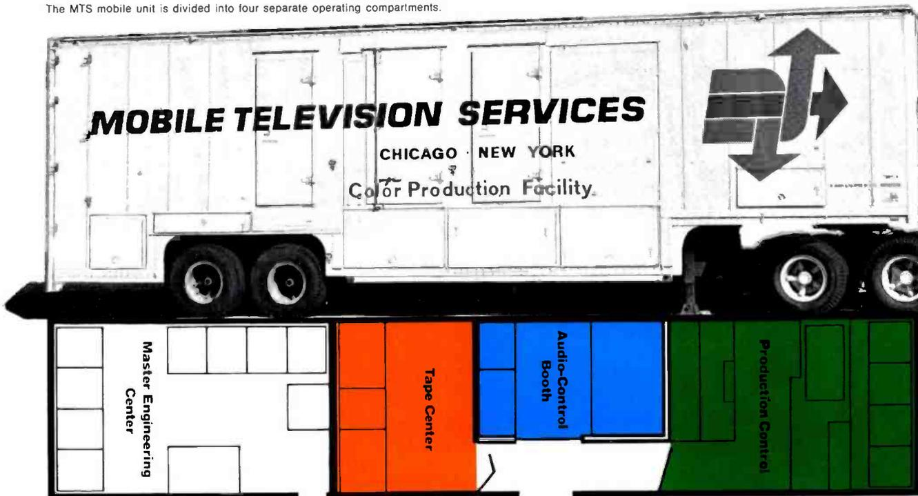
Mobile Television Services' 40-foot mobile unit is a fully equipped video production center.
