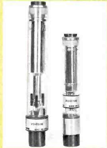
Size comparison between a 30 mm PbO and the one-inch lead oxide type tube used in TKP-45. Advanced video amplifiers in the TKP-45 camera bring signal-to-noise performance of the smaller tube to be equal with the larger tube design.
