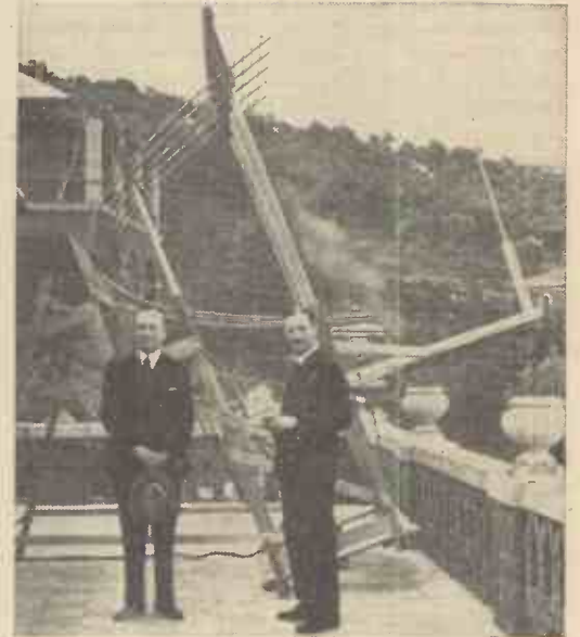
1932: Return to ultra-short waves. Aerial and reflector for transmission of 57-centimetre waves
