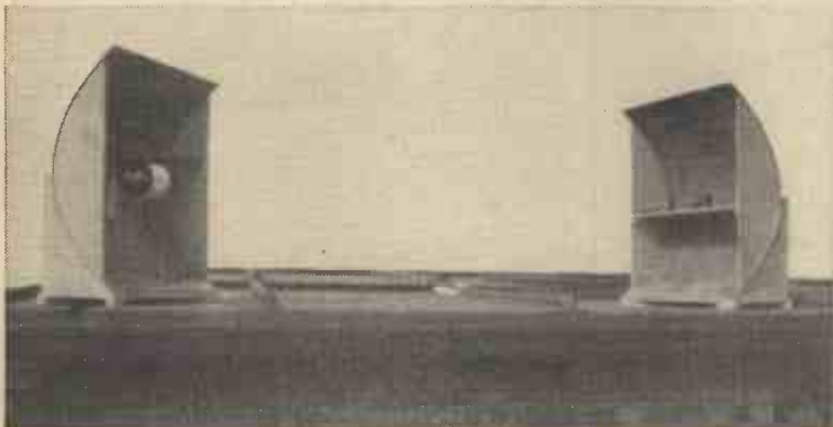
1895: Replicas of experimental short-wave beam transmitter and receiver used by Marconi at his father's house in Bologna
