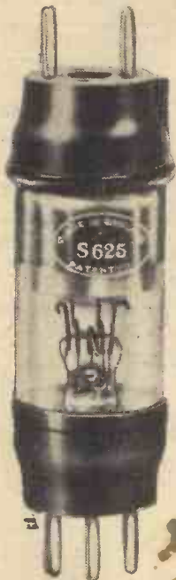
Fig. 9—First screened-grid valve—Marconi S.625
