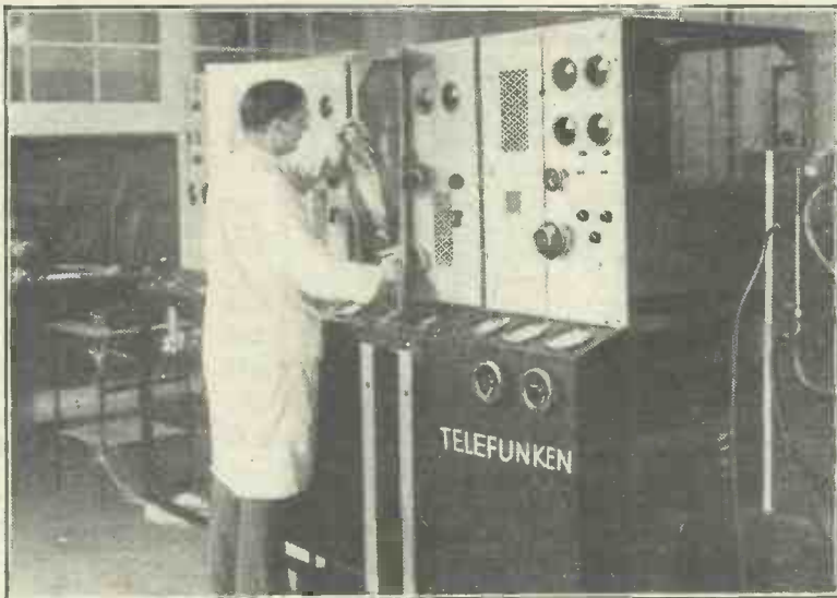
The new 15kW transmitter for the Berlin ultra-short-wave station
