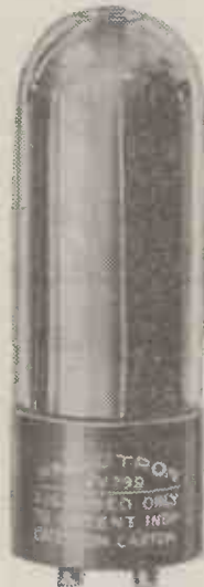
This is the standard .06 ampere American valve on the old type of base.
