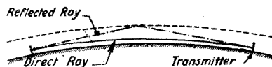
Fig. 1.—Fading may be explained as due to interference between a direct ray and a secondary ray reflected from the upper atmosphere.
