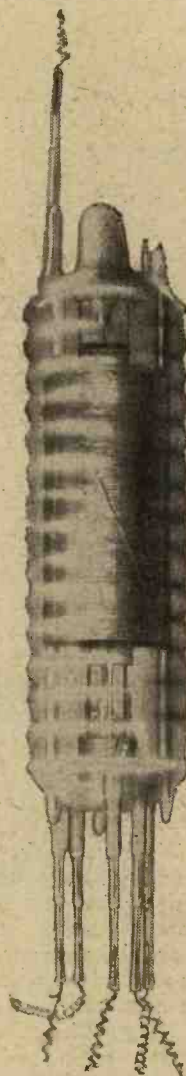
One of the high-power silica valves made by the Mullard Wireless Service Company, Ltd., to the design of H.M. Signal School, Portsmouth.
