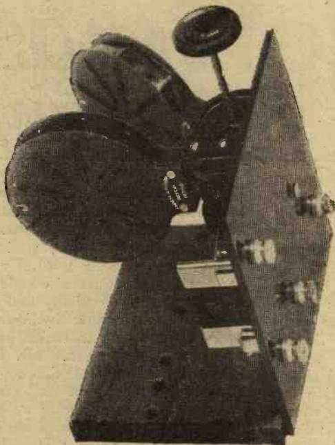
Terminals are mounted on the vertical panel for convenience in connecting the unit to the receiver.
