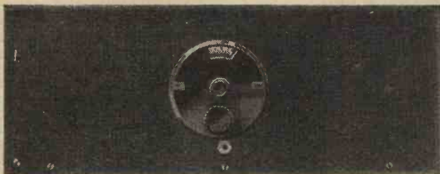
The controls on the front panel of the receiver consist of one tuning knob, and a jack by means of which the filaments are switched on when the telephone plug is inserted.
