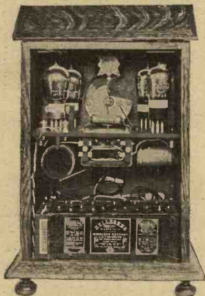
The anode and grid batteries are placed inside the cabinet.
