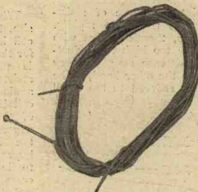
The H.F. resistance of fine wire windings of the types illustrated may be quite low so long as the coil is correctly proportioned.
