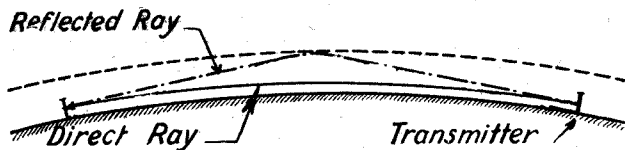
Fig. 1.—Fading is thought to be due to interference between two waves arriving at the receiver by different routes.
