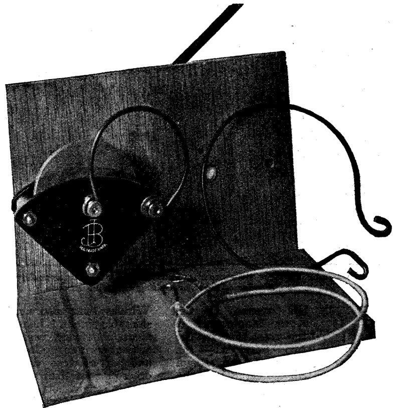
A wavemeter of the type described can be very simply made up, the only parts required being shown here, changes in the wavelength range to be covered being effected by the use of different sizes of coils.
