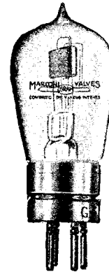
The Marconi general purpose bright emitter valve, type R.5.V.
