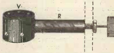
Fig. 2.—A back-of-panel valve holder incorporating a filament resistance.
