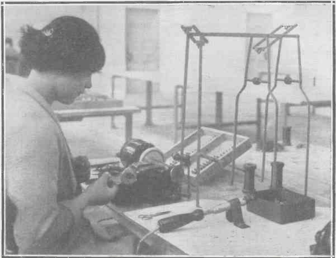
An interesting operation. Winding the fine enamelled wire on to the magnets of telephone ear-pieces at the Brandes factory. A high-speed motor is used and the tension is carefully controlled by the operative.
