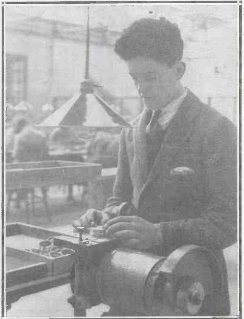
Grinding the faces of telephone pole-pieces in the Brandes factory.
