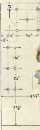
Fig. 2.—Theoretical circuit diagram of the instrument. It will be noted that the positive side of the L.T. battery is earthed instead of the more usual method of earthing the negative side. Fig. 3.—Showing position of drill holes and dimensions of panel. A blue print of this figure is obtainable from the offices of this journal.
