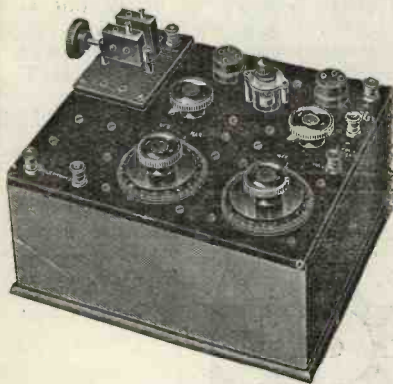
A valve-crystal receiver (ST100) by Radio Instruments, Ltd.
