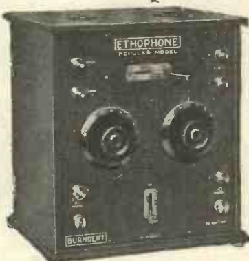
No. 510 W.A.—Ethophone Popular Model. A 2-valve highly efficient long distance receiver, complete with self-contained High Tension Battery, Accumulator, Telephones and Aerial Equipment. Price £18 10 0 To which must be added Broadcast Tax £ 17s. 6d.
