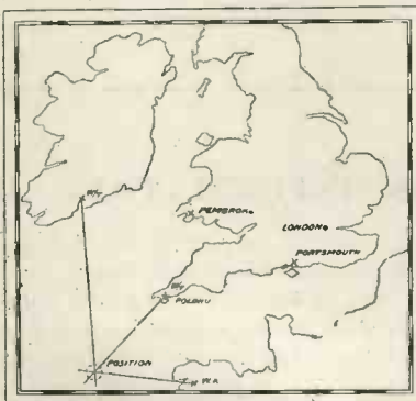
Fig. 4—Showing how the position of a ship or aeroplane is determined by cross bearings of coast stations.
