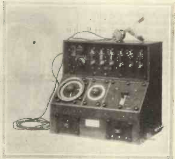
The Marconi Type 11 B marine direction-finder, which was exhibited recently at The Shipping and Engineering Exhibition.
