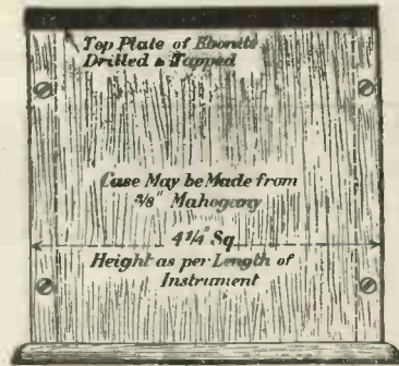
Fig. 6.—Case for containing the plates of the condenser
