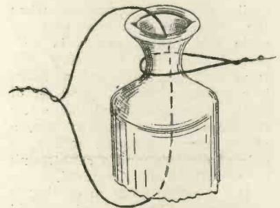
Fig. 8.—The "broken-bottle" insulator.
