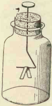
Fig. 2.—Simple form of gold-leaf electroscop.
