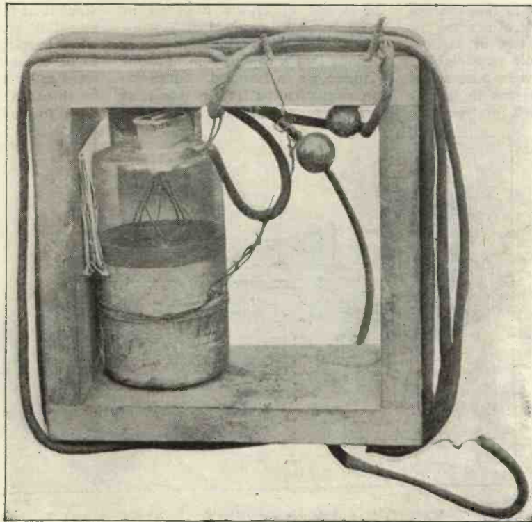
Fig. 1.—Illustrating the first Marconi short-wave tuned transmitter.
