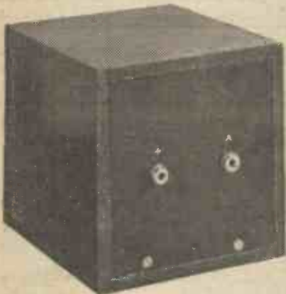
The loud-speaker terminal on the set which goes to H.T.+ should be connected to the left hand socket in this photograph.
