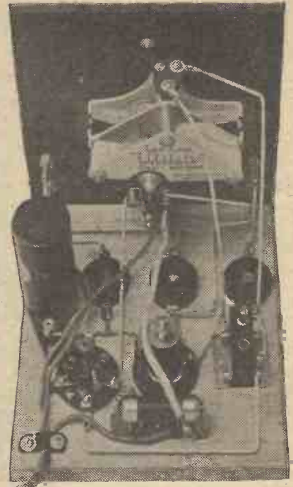
The wiring requirements are few, as may be gathered from this photograph. The flex which forms the tapping on the coil may be seen hanging over the resistor.
