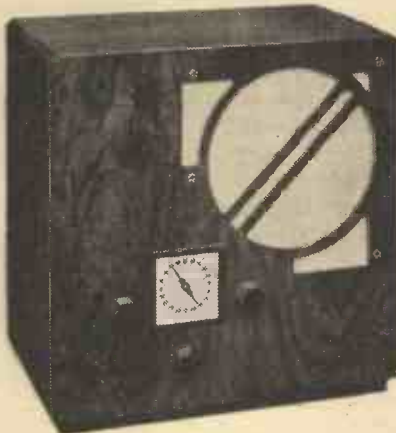
Here is the Model 431, a 3-valve battery receiver made by Kolster-Brandes.
