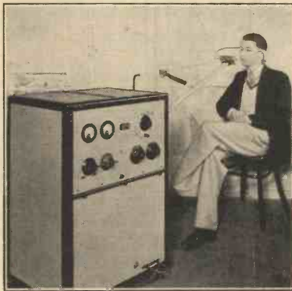
A Marconi ultra-high-frequency therapy set. Apart from its uses in medical treatment, this apparatus is specially suitable for investigating the effect of high-frequency currents on bacteria cultures. The range of wavelengths available with this particular set range from 8.5 to 2.6 metres.
