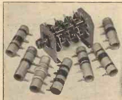
The Bulgin multiple coil chassis and the coils which are used in conjunction with it. Only five of them are mounted at any one time.
