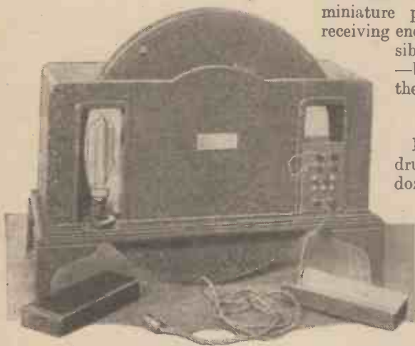
One of the early Baird televisions which were designed for the reception of 30 line television broadcasting such as that which the B.B.C. has been transmitting for the past two years or so.
