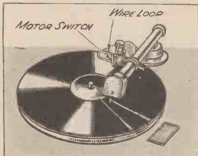
The addition of the wire loop makes it possible to start the motor by simply moving the pick-up arm momentarily away from the record.
