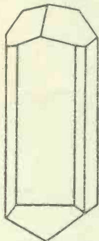
Fig. 1. A typically asymmetrical crystal. It is tourmaline, one of the first crystals to be found exhibiting piezo-electric qualities.
