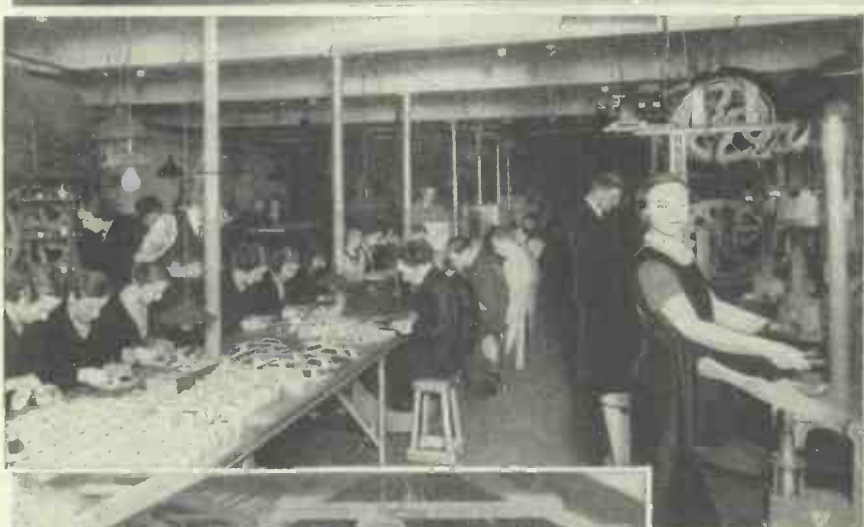
Top left: Winding the output transformer. Above: How the field magnets are magnetised. Left: An assembly bench, along which the speaker progresses from stage to stage. Bottom: A plating room where magnets are given a coating of cadmium.
