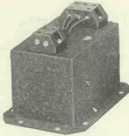
The Trix suppressor for use at the meter. It is inserted in series with the mains, the connector blocks on top being employed for this purpose. The suppressor is housed in a metal case.
