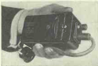
This is the neat Belling-Lee suppressor for connecting in series with the set's mains lead.
