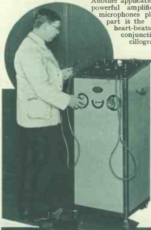
The use of high-frequency and other electrical currents for medical purposes is quite common these days. This photograph shows a Marconi valve diathermy set which is suitable for both therapy and surgery.
