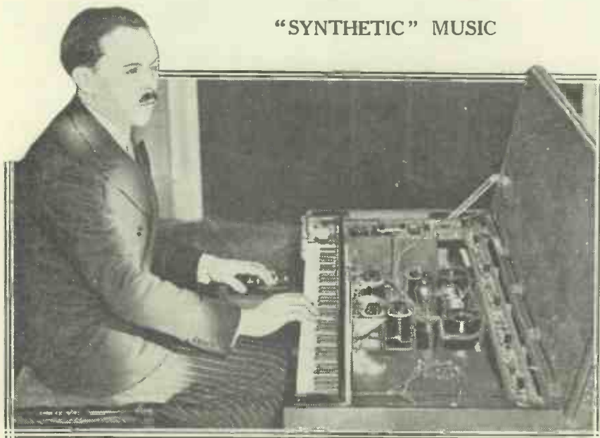
This is an electronic organ of quite a different kind. It relies on tuned circuits for its notes and does not make use of any revolving discs.
