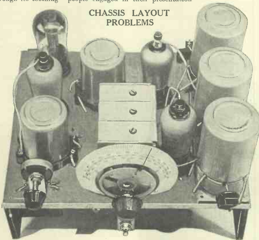
The extent to which the chassis layout of a set governs the positions of the controls is clearly indicated in this photo. It will be seen that the greatest difficulty in the way of any elasticity in arranging them is the ganging of condensers and coils, which is necessary in any modern design.
