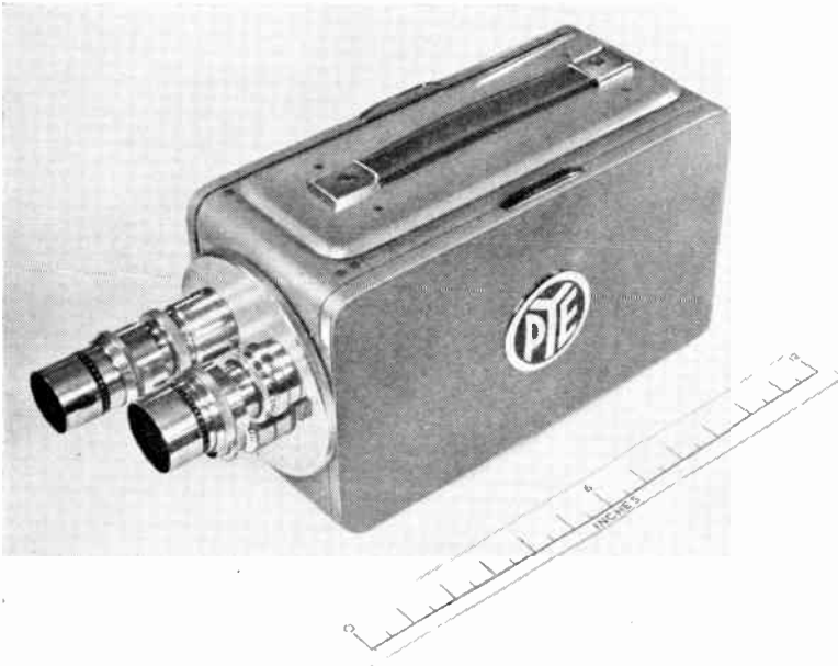
Fig. 51—A camera intended for industrial use and using a photo-conductive tube (Staticon)
