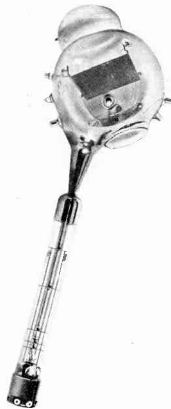
Figs. 19 and 20—An iconoscope; this particular tube is a standard Emitron
