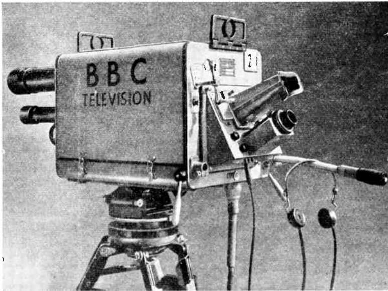
Fig. 122—Rear view of image iconoscope camera showing viewfinder hood
