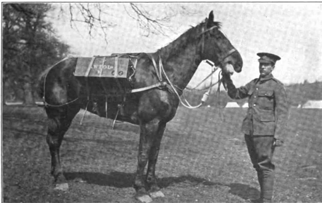
Digitized by Google The Instrument Load, Showing the Manner in Which the Transformer is Secured to the Saddle. Original from HARVARD UNIVERSITY
