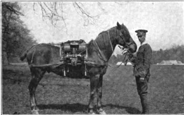
The Gasoline Engine is Fitted to a Specially Adapted Saddle Frame.
