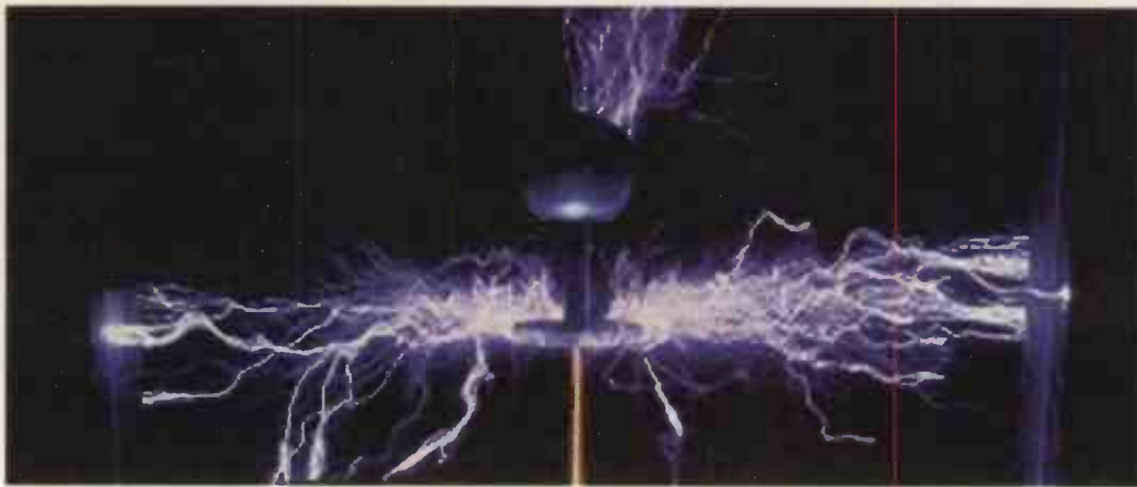
Very high voltages are generated by this modern version of Tesla's coil – page 190.
