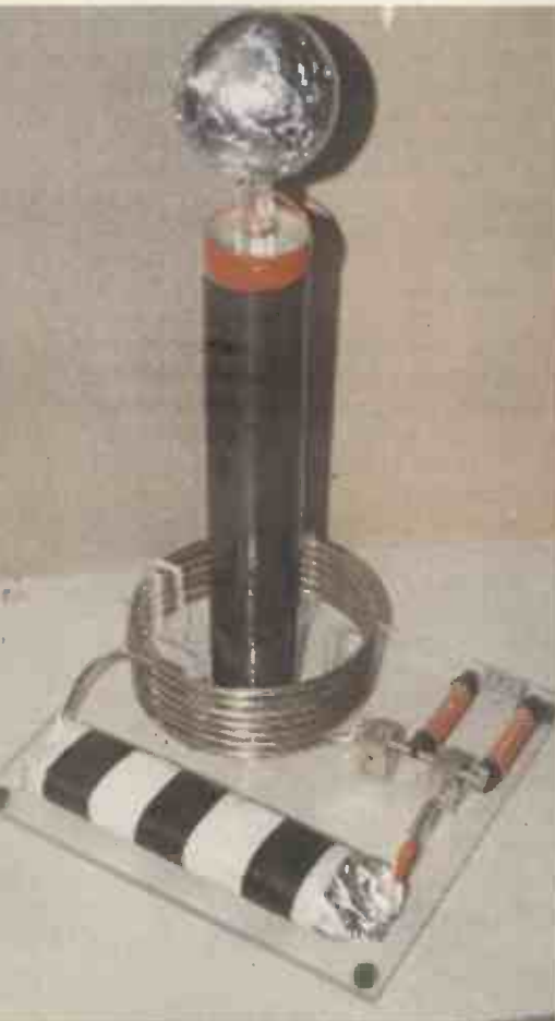
The finished Tesla coil ht generator can be seen here with custom-built capacitor, and coil former containing both primary and secondary coils.
