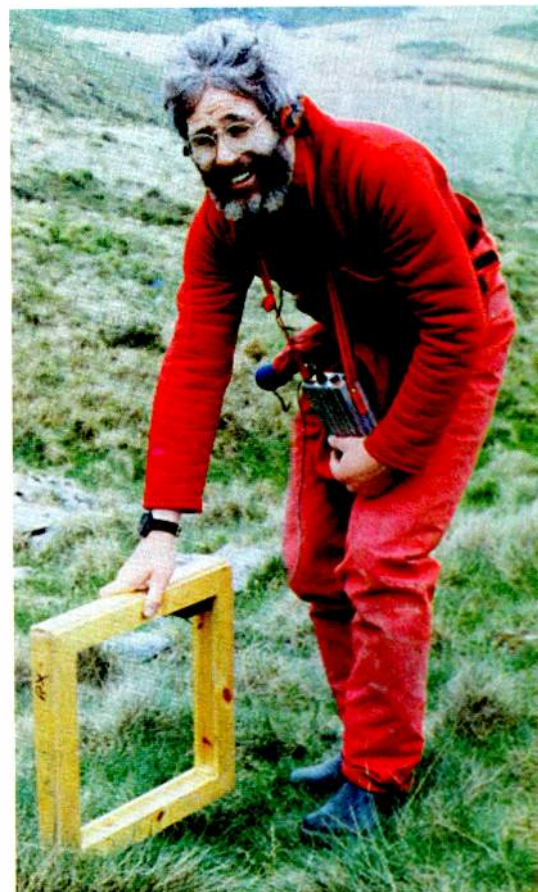
Steve Laugher, G7LYN, locates an underground beacon using an 874Hz receiver.
