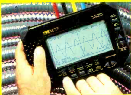
Dual channel operation allows relative timing of signals to be observed.
