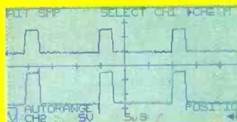
Dual channel operation allows relative timing of signals to be observed.
