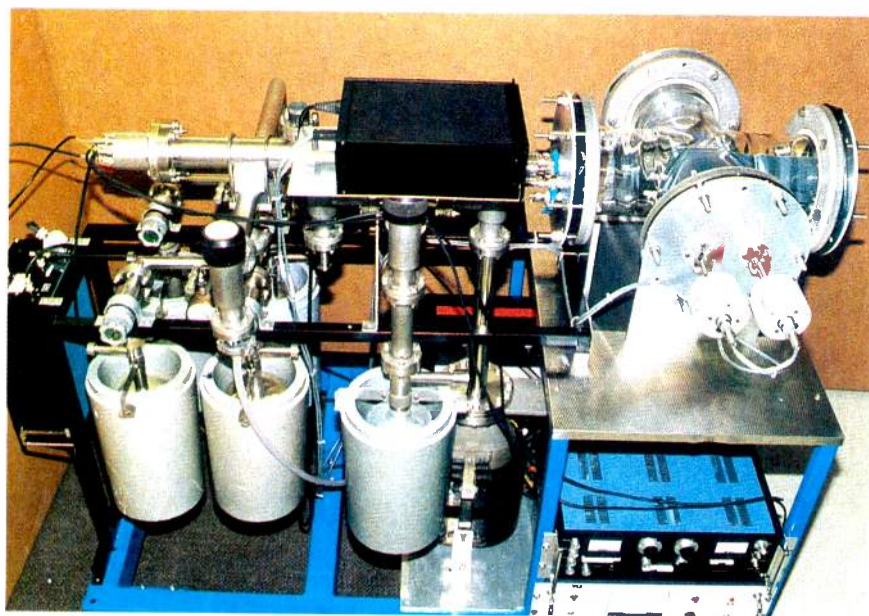
Intentionally gas-filled components in orbiting satellites have been known to leak their gas into the surrounding void, causing failure. Researchers at Kent University are using the vacuum equipment shown here to research this problem – the inverse of 'soft' thermionic valves.
