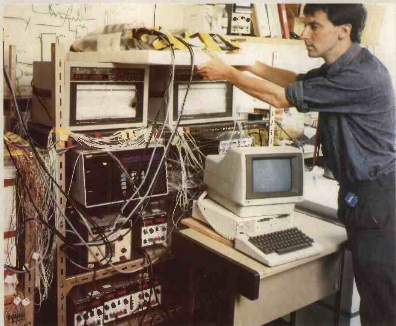
Inconclusive search: Dr Derek Craston examines data logging equipment used in the calorimetric measurements on 24 cold fusion cells. Despite closely matching the original conditions which were said to have produced excess heat, AEA Harwell's researchers were unable to duplicate the results.
