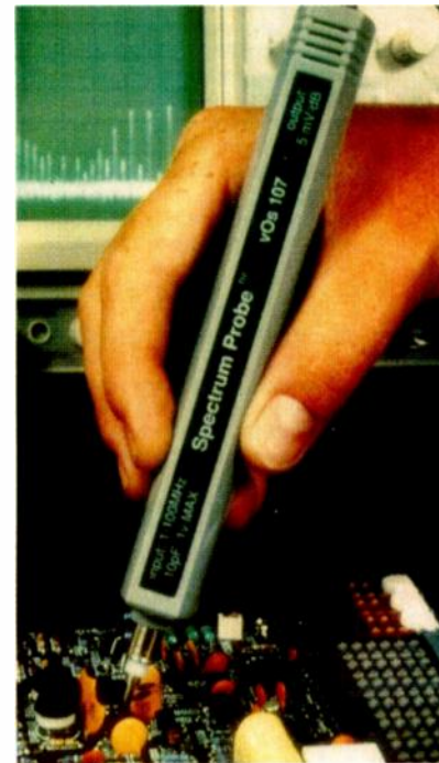
Getting the point: the Spectrum Probe converts a standard scope into an EMC sniffer.
