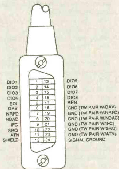
GPIB connector showing how each line is assigned.
