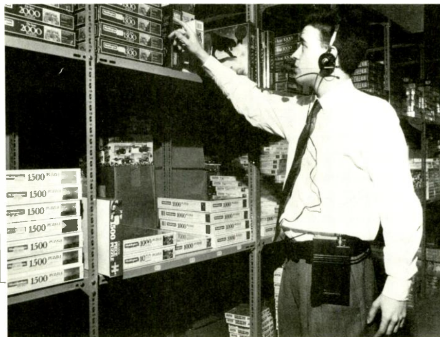
Personal stocktaking: this belt worn data logger from Marconi provides both prompt questions and analysis of the spoken answer.
