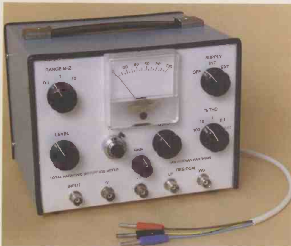
Fig. 2. Completed battery-powered THD meter, showing the flying supply lead, via which the unit can alternatively be powered from an external source of \pm 15 to 18V dc.
