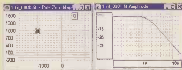
Fig. A. Pole-zero map with a complex pole at -1000, j1000 . It has a companion pole at -1000, -j1000 , not shown. This represents a second-order filter providing a low-pass response shown on the right.
