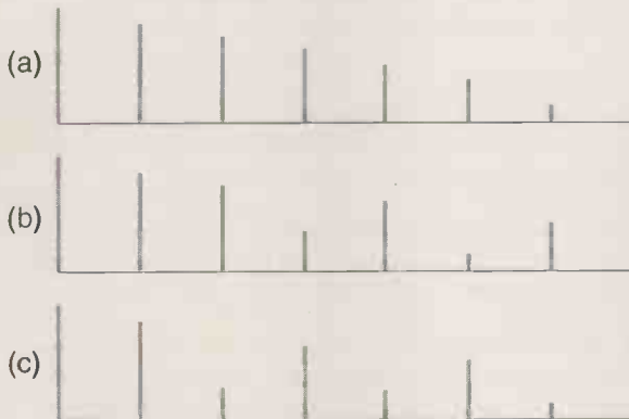
Fig. 4. Pitch recognition is based on the pattern of harmonics rather than their levels. Spectra a), b) and c) all have the same pitch.
