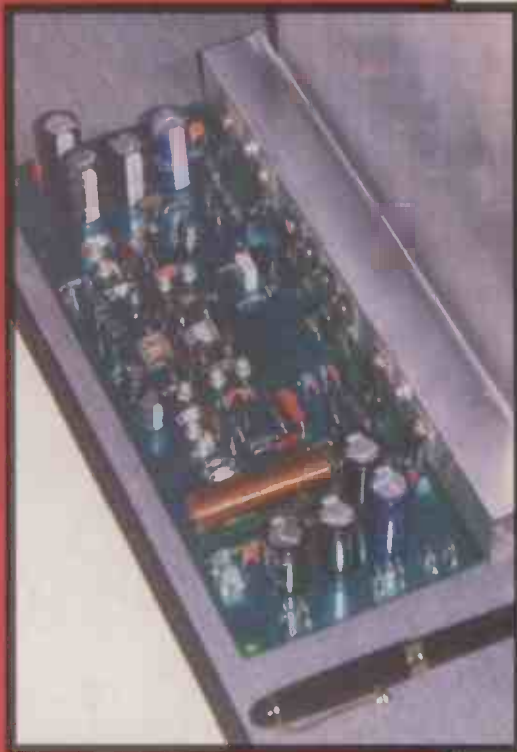
Giovanni's high-performance power amplifier mounted on its heat sink.
