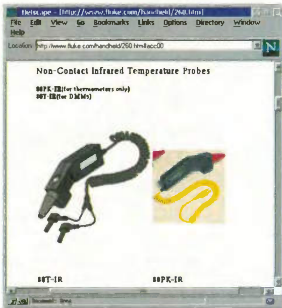
Fig. 4. This low cost non-contact hand-held infra-red probe could be ideal for measuring the temperature rise of your plastic IC package.
