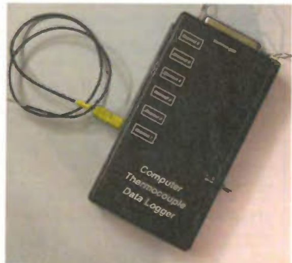
Since the logger is based on CMOS devices, it can be implemented compactly and operated from a 9V battery.
