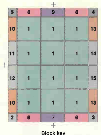
Fig. 1. Block diagram of a 3-by-4 ccd showing the arrangement of the basic building blocks.
