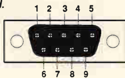
(a) 9-pin male socket viewed from the back of the computer
