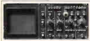
PHILIPS PM3217 (This is a proper scope) Dual Trace 50MHz Delay Sweep Incl 2 Probes £400
