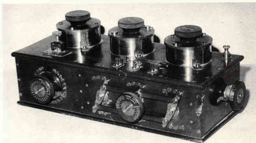
Photo 3. Multiple tuner from circa 1909 was used to tune receivers relying on magnetic detectors.
