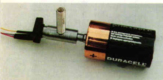
Fig. 3. Mkl fixture used for monitoring pressure in the cell during charge incorporated a sensitive electronic pressure transducer. Although more sensitive than the mechanical pressure gauge, this version still showed no significant rise in pressure – as chart Fig. 4 illustrates.
