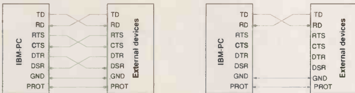
Fig. 4. RS232 pin connections between pcs and external devices.
