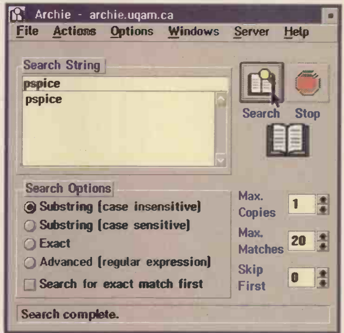
Fig. 1. Using Archie to search for the location of 'P Spice' software file. Search for 'P Spice' using the Archie server located at 'archie.uqam.ca.' in Canada. Note the 'aid memoir' display of used search strings.
