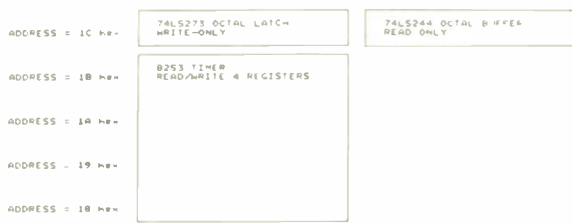
Fig.3. This address decoder memory map can be implemented in a pal without the peculiarities such as address redundancy shown by the TTL implementation of Fig.4.
