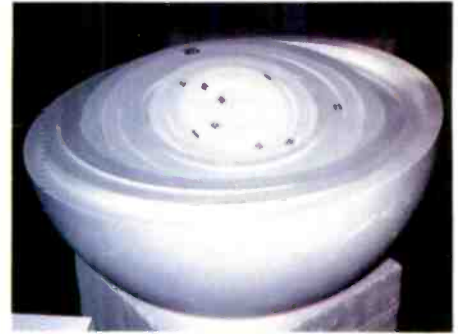
Fig.3. Half a Luneberg lens, showing the shells.
